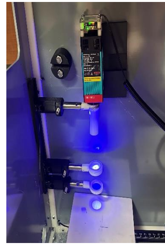
Figure 7: Early Stages of Laser and Lens System. The laser module is on top followed by the aspheric lens and beam expansion pair. The beam is too large and is onset a white screen
